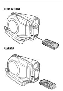
Point the controller at the camcorder's remote sensor when you press the buttons.
