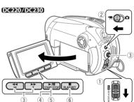
Move the power switch to ON, then slide it down toward MODE and release it to set the camcorder in PLAY mode.
