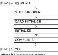
\* Press ((ET)) to cancel the complete initialization while it is in progress. All the image files will be erased and the memory card can be used without any problem.
